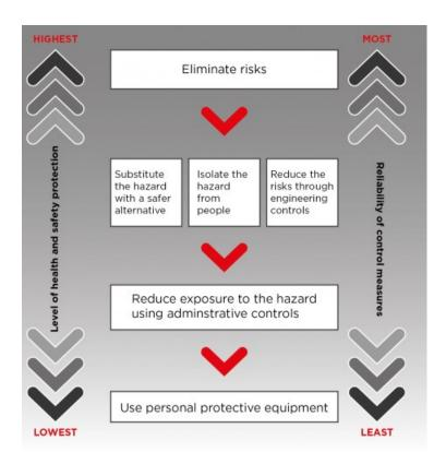
Figure 3: The hierarchy of control measures.
