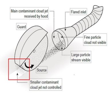
Figure 5: Operational view of local exhaust ventilation.
